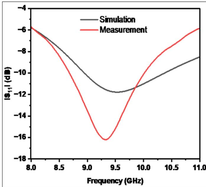
Figure 9. Return loss of the simulated and measured results of the PAC thick film MPA
