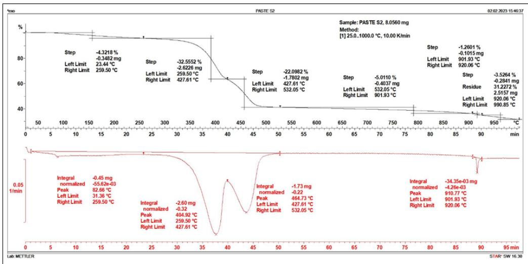
Figure 8. TGA measurement of PAC paste thick film
