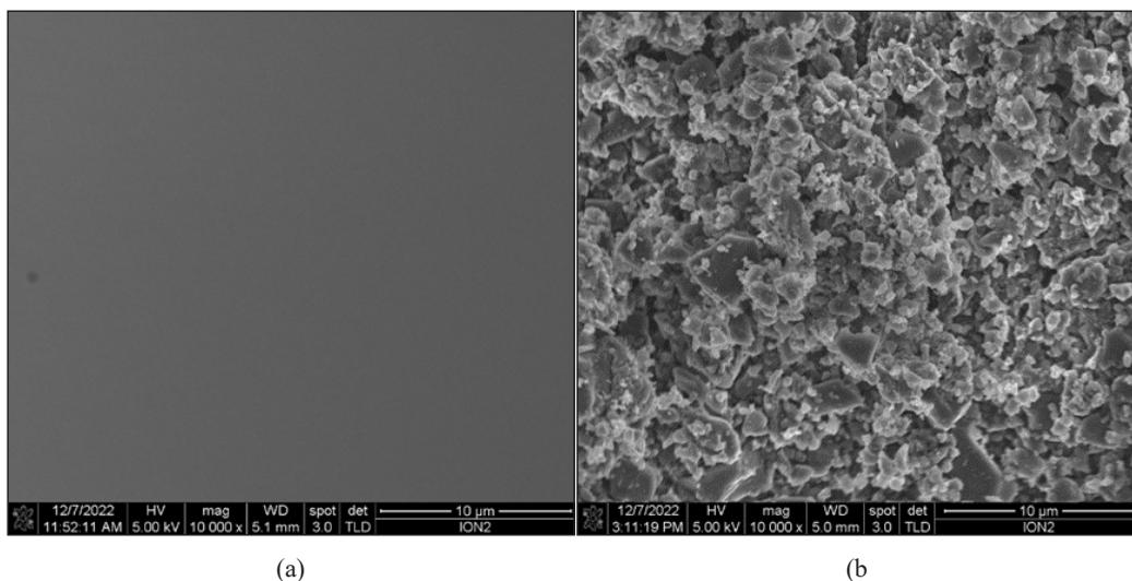
Figure 6. Morphology of PAC film (a) at room temperature and (b) firing at 300 °C
