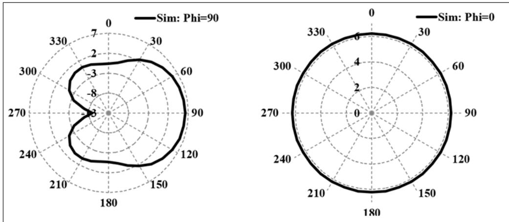
Figure 10. The simulated 2D radiation pattern of the proposed antenna
