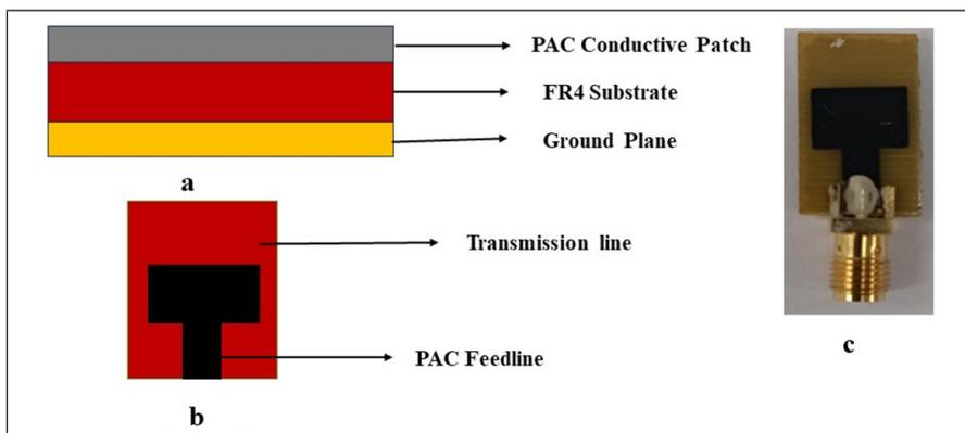
Figure 4. MPA structure: (a) view from the side, (b) view from the top, (c) fabrication prototype
