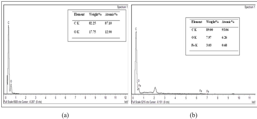
Figure 7. EDX of PAC film at (a) room temperature and (b) at firing temperature at 300 °C
