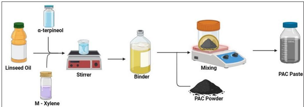
Figure 3. Formulation of organic binder and PAC paste thick film for screen printing
